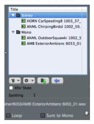
7. Transfer your mono files by highlighting the mono folder. Click the sum to mono button and then transfer the files with the green arrow button.
