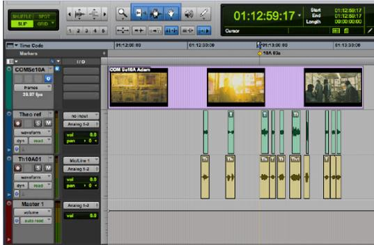
Here is a finished ADR session with the reference (production) dialogue and the ADR. Listening to the reference and ADR clips together reveals that some of the ADR is almost exactly in sync and some is noticeably off. Thanks to a remarkable bit of software called VocAlign, making the timing of ADR match the timing of production recording is (usually) very simple.
