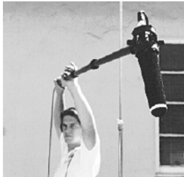
An overhead mic will pick up sufficient sound effects, footsteps, and hand-prop noise to give the soundtrack a full texture. Because the faces are closer to the mic, dialogue will dominate the track, but other sound effects will still be audible.
