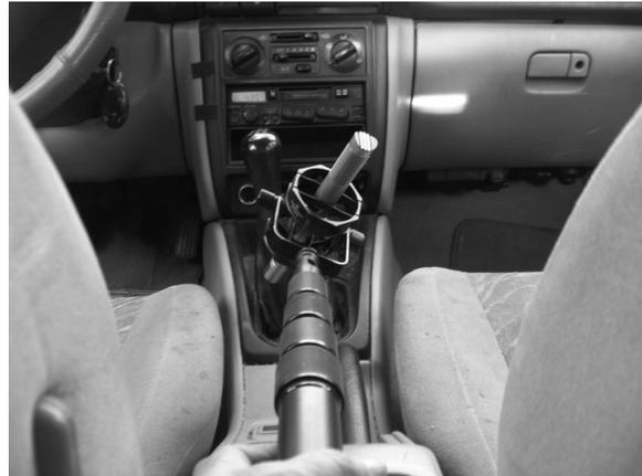
**ADVANTAGES:** the mic is completely isolated from the car's mechanical vibrations, you can get it closer to the actors' mouths than with the CUB-01s, you can rotate left and right to follow the dialogue.
